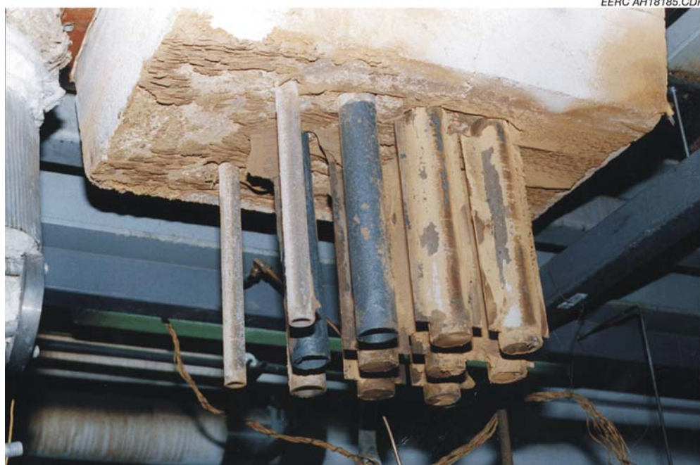
Figure 9. Photograph of the CAH tube bank used in support of Tests XCEL1–XCEL3.
