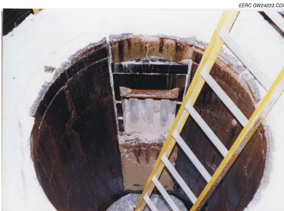
Figure 22. Photographs of the slagging furnace interior after high-density refractory curing (top) and after 751 hr of solid-fuel firing (bottom).
