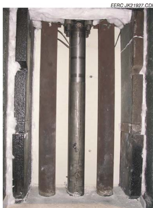
Figure ES-2. Photograph of the HTHX, modified to include a center tube of MA956 alloy, prior to Test SFS-XCEL1-0303.
