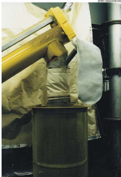
Figure 5. Photograph of the grain auger discharge and top of the biomass feed hopper.
