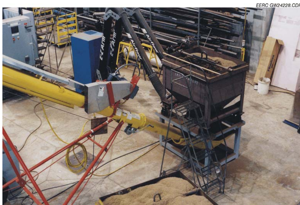
Figure 4. Photograph of the biomass charge hopper and grain auger supporting the biomass feeder.
