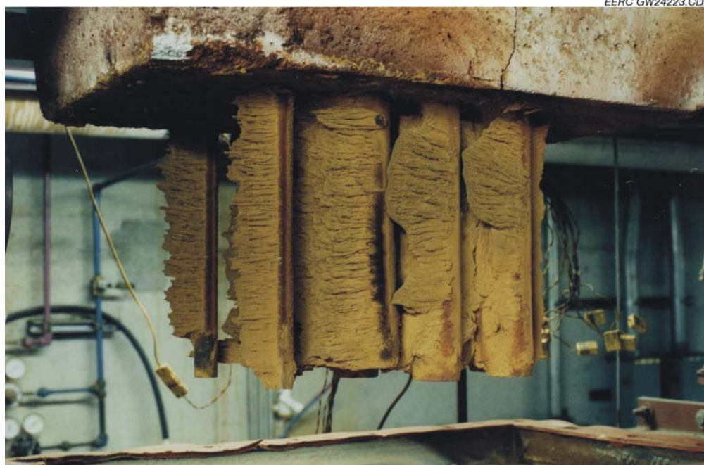
Figure 39. Photograph of ash deposits on the CAH tubes following Test SFS-XCEL1-0303.
