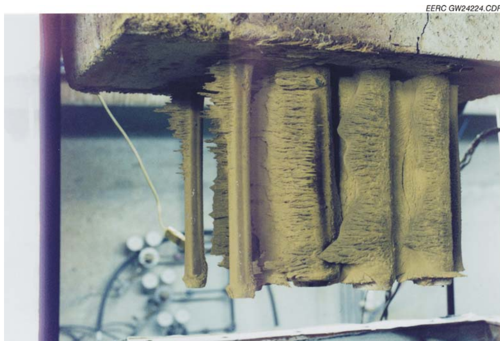
Figure 41. Photograph of ash deposits on the CAH tubes following Test SFS-XCEL2-0403.
