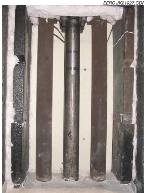
Figure 7. Photograph of the HTHX, modified to include a center tube of MA956 alloy, prior to Test SFS-XCEL1-0303.
