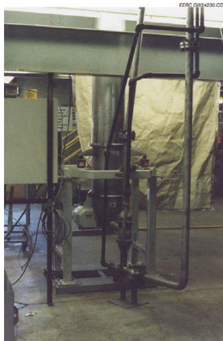
Figure 6. Photograph of the biomass loss-in-weight screw feeder.
